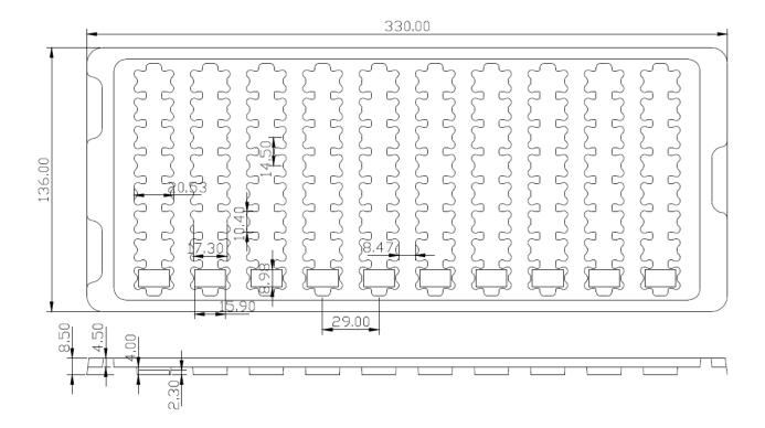
The tray is designed for direct use on a SMT automatic machine.
