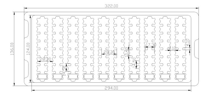
The tray is designed for direct use on a SMT automatic machine.
