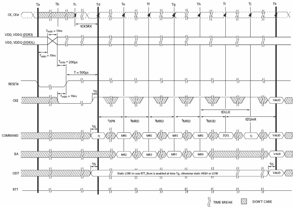
Note : From time point Td until Tk, NOP or DES commands must be applied between MRS and ZQCL commands
